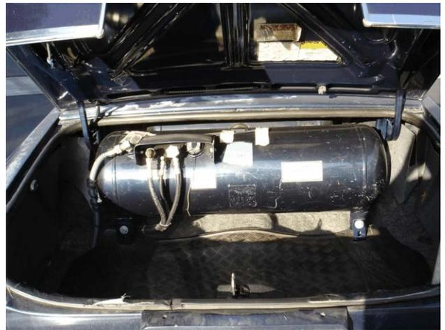
Trunk installed LPG manifold tank.
